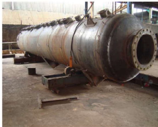
BACK PRESSURE VESSEL
